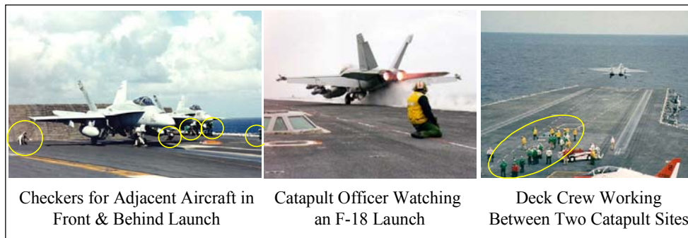
Figure 6: Photos of Deck Crews at Work in Close Proximity to Jet Noise
